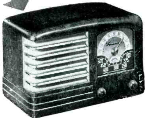
FARNSWORTH MODEL CT-43 . . . A two-way winner. Cabinet-enclosed battery, 4-tube Superheterodyne. Permanent magnet dynamic speaker. Standard and police broadcasts. Automatic volume control. Convertible to 5 tube AC-DC by adding 117Z6GT tube. Operates from any standard make power pack. Two-tone mahogany plastic cabinet with bronze finish grille. Size 12" long, 7 \frac{3}{8} " high and 7" deep.
