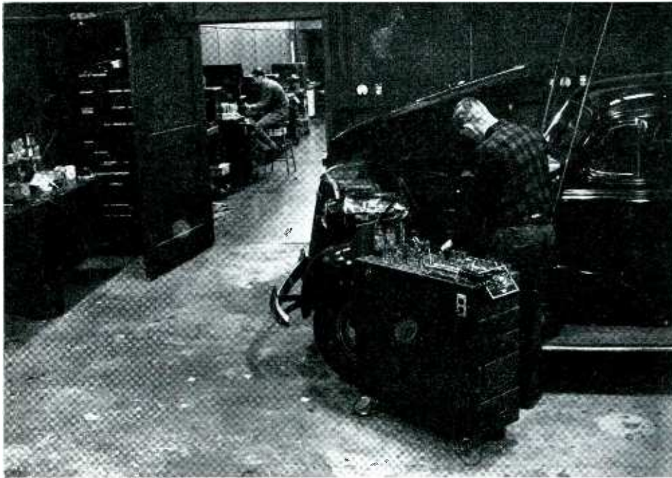
BENCH ROLLED TO CAR —Clever combination test instrument and parts supply trucks used by Milt and Harold Kidder of Madison, Wisconsin step up service
