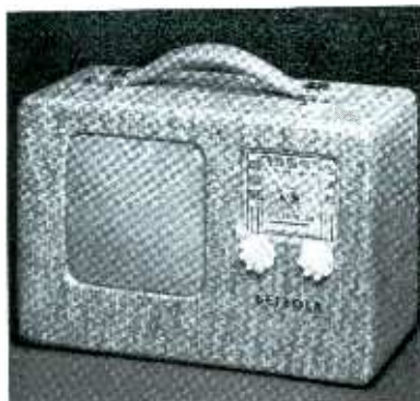
DETROLA 3-WAY PORTABLE radio, model 383, has 5 tubes and operates on ac-dc or battery. Tunes 540 to 1600 kc. Compact, wood cabinet with covering of aeroplane cloth of neutral color. Measures 7½ high, 11 wide, and 5 inches deep. Weighs 12 lbs. List price $19.95. Detrola Corp., 1501 Beard Ave., Detroit, Mich.
